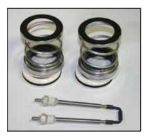
The seals are lubricated by a large capacity oil-filled chamber and protected from water leakage into the chamber with a two-conductor probe that senses and alarms water entry well before any water can enter the motor housing.
